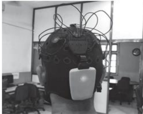
Fig 2. Device used for recording EEG signals of the subjects
